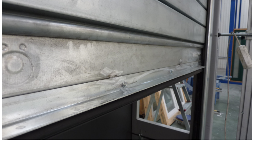
Image 11: Test sample No. 11/03-A091-P1 reinforced end profile
