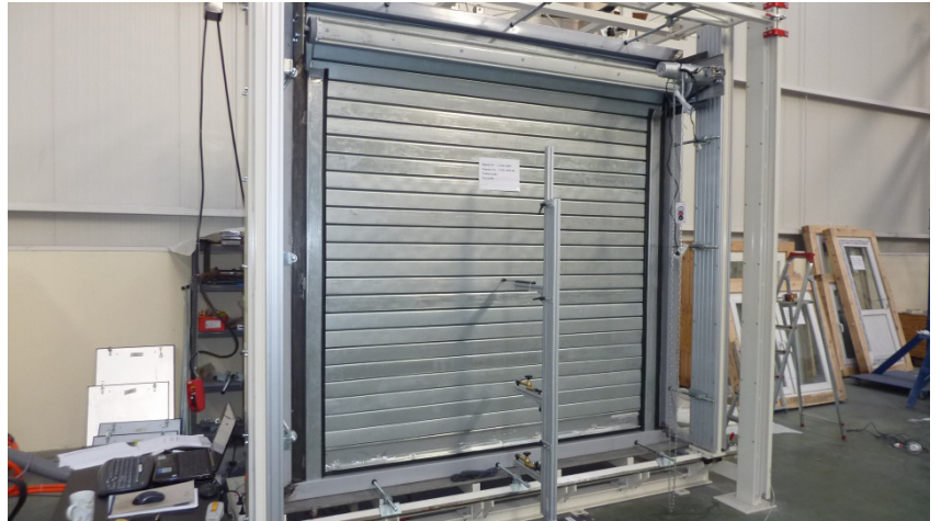
Image 8: Test sample No. 11/03-A091-P1 Deflection gauge placed on the sample for wind load testing
